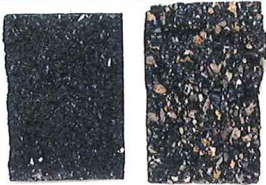
Left, HMA sample with no moisture damage Right, HMA sample with moisture damage. Notice the amount of uncoated aggregate on the right?
